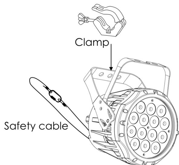
The Spectral can be placed on a flat stage floor or mounted to any kind of truss with a clamp.
