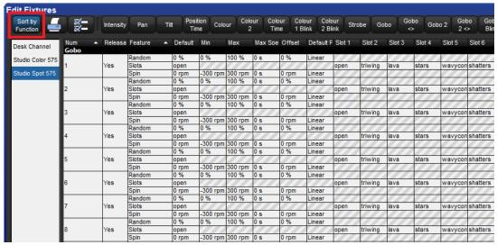
Figure 5.11. The Edit Fixtures window sorted by Function
