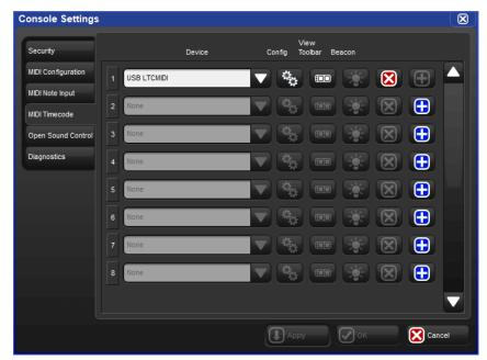
Figure 21.4. The MIDI Timecode pane of the Console Settings window
