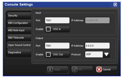
Figure 22.1. The OSC pane of the Console Settings window
