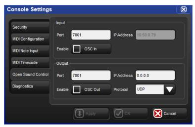
Figure 22.2. The OSC pane of the Console Settings window
