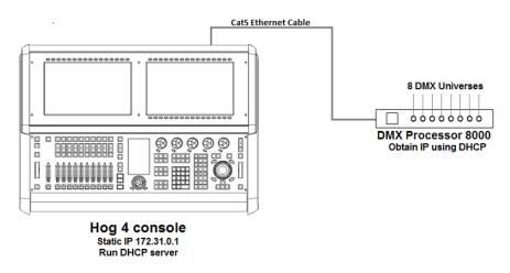
**Example B:** The console is a DHCP server, and all other nodes obtain an IP address from it.
